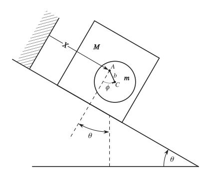
The axle A passes through the center of mass of the block of mass M. The disk has a mass m. The disk is pivoted on an axle through A at a distance b from the center of the disk C. I is the moment of inertia about C. The generalized coordinates are X and  $\phi$ ;  $\phi$  is measured from the line through A which is perpendicular to the plane.  $\theta$  is the angle made by the incline with the horizontal.
