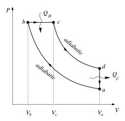
(a) Show that, for a quasistatic reversible engine undergoing this cycle using an ideal gas, the ideal efficiency e is given by:
