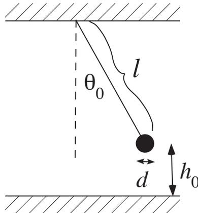
A pendulum consists of a spherical bob of mass  $m$  and diameter  $d$  suspended by a rigid, thin wire of length  $l$  and negligible mass. The initial position of the bob is such that the wire makes an angle  $\theta_0$  with the vertical. The local acceleration due to gravity is  $g = 9.8 \text{ m/s}^2$ . The bob is released from rest. Due to air resistance, it does not return exactly to its starting height  $h_0$  after one full oscillation.
