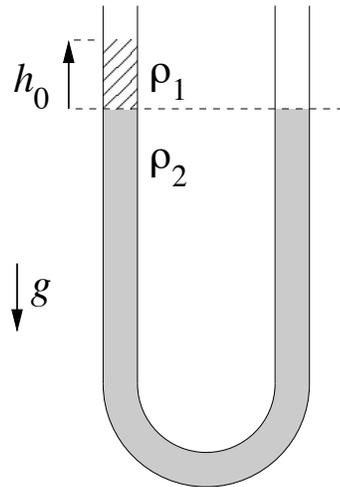
Consider two immiscible fluids of unequal densities ( $\rho_1 < \rho_2$ ) in a fixed, U-shaped tube, open at each end. (For example, fluid #1 might be oil, and fluid #2, water.) The fluids are poured into the tube, then released from rest, starting from the initial geometry depicted in the accompanying figure.
