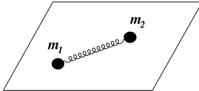
A massless spring, of spring constant  $k$  and equilibrium length  $\ell$ , connects two point masses,  $m_1$  and  $m_2$ . Each mass is able to slide without friction in any direction along a smooth horizontal surface, as shown in the figure.
