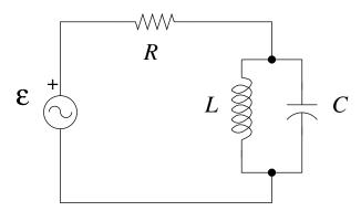
In the circuit above an ac voltage source  $\varepsilon = V_0 \sin \omega t$  is connected in series with a resistor (resistance R) and a parallel inductor (inductance L)-capacitor (capacitance C) network.
