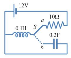
After the switch S has been in position a for a long time, it is moved to position b. What is the maximum voltage across the capacitor?
